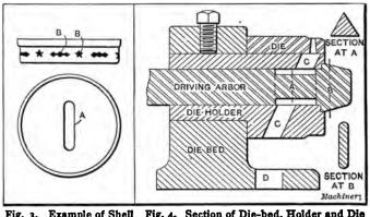
Fig. 3. Example of Shell Fig. 4. Section of Die-bed, Holder and Die to be Perforated for Perforating Shell shown in Fig. 3
